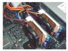
Dual PL-P3/SMPs, installed and connected.
